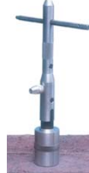
5. Attach tool. Turn clockwise to remove anchor.
