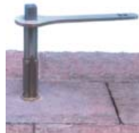
1. Insert tap in pop-up shell to create threads (For threaded shell proceed to 2)
