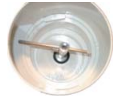
Hold plugs in place for vacuuming
